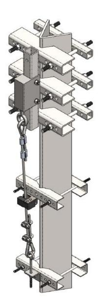
Universal angle leg head adaptor bracket with fasteners for 4" to 8" legs
