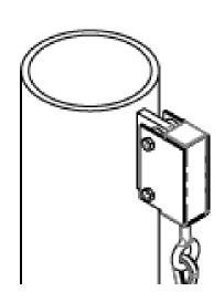
Vertical tab mount (includes spacer sleeves)
